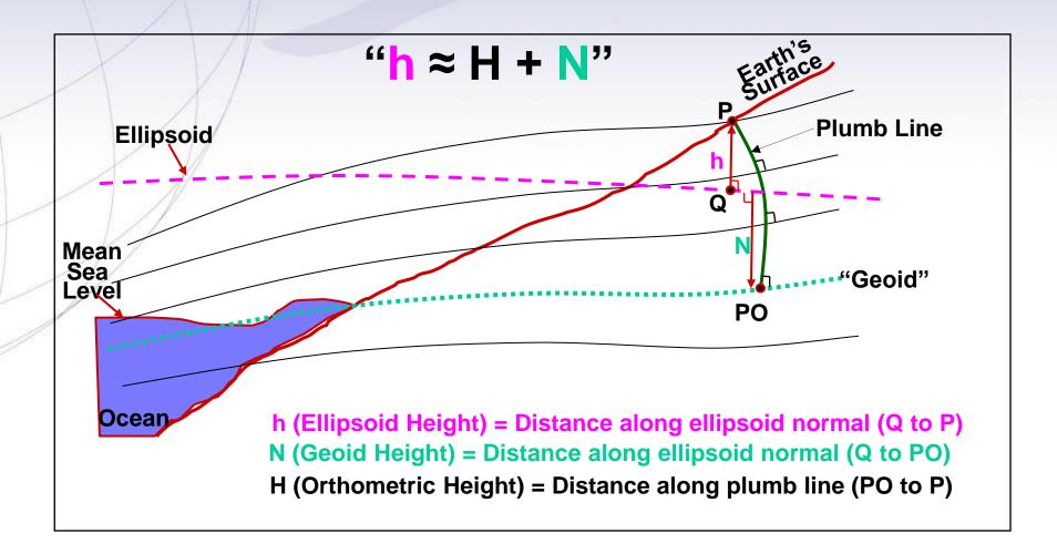
Hybrid Geoid Height Models (e.g., GEOID09) are determined from Gravimetric Geoid Height Models (e.g., USGG2009) and Conversion Surfaces based on GPS on BM data
