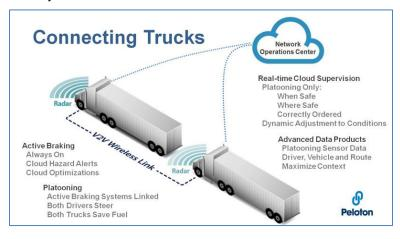
Figure A-10. The City of Columbus may partner with Peloton to deploy two-truck platoons along Alum Creek Drive to reduce congestion and increase capacity.
