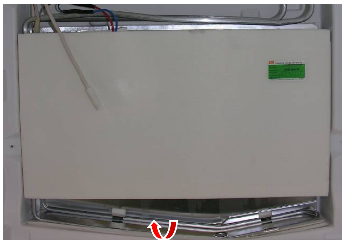
Fig. 5.3.1/ 2 Swinging out the evaporator module
