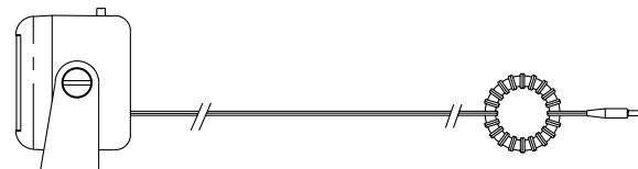
Figure 8. Power lead suppression.
