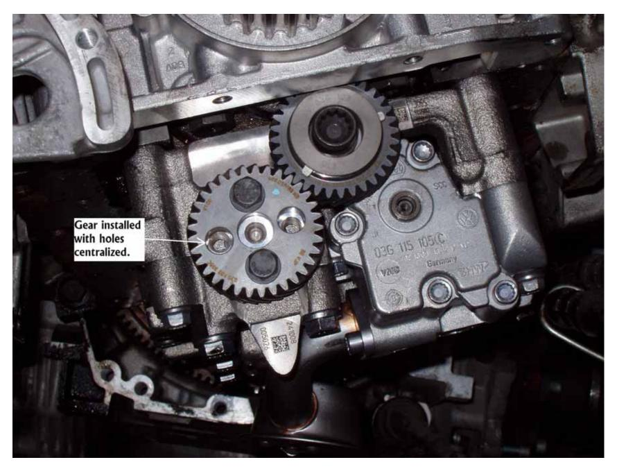
Install bolts N 911 213 01 in balance shaft gear and tighten to 20 Nm plus ¼ turn.
