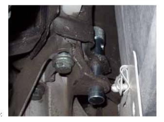
It is recommended that you use SST MOTOOL-GH0002 on a support under the oil pan to lift the engine a little higher before lifting the subframe into position. This makes it easier to lift the subframe into position without the weight of the engine resisting your efforts.
