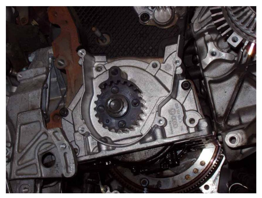
Note that the intermediate gear has a coating. **Do not damage this coating** while handling the balance shaft module.
