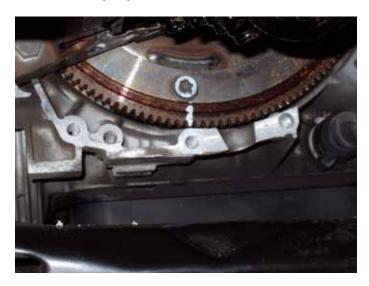
Remove the sealing flange from the front of the engine. Clean off old sealant from flange and engine block. Remove old crankshaft seal.
