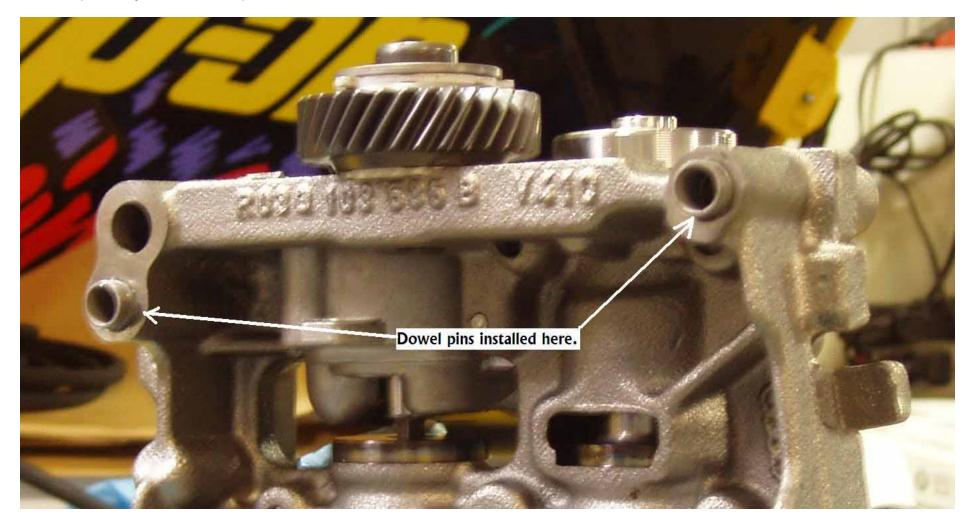
Make note of the position of the thrust washers on either side of the intermediate gear attached to the module. These have ears. The ears of the washer between the gear and the module fit into depressions on the module body.
