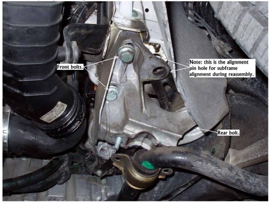
Remove bolts from subframe on either side of the transmission mount. Repeat for other side.
