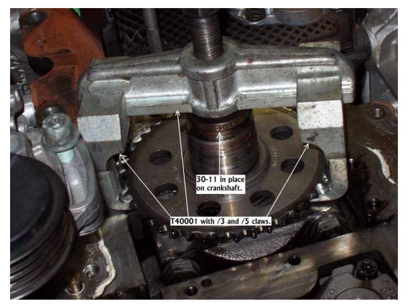
Slowly turn the screw to apply a pulling force on the sprocket. We have never been able to pop one off the crankshaft in one piece. The sprocket will break. Lightly grease the end of the crankshaft. Remove crankshaft bearing cap #1. Use an air hammer with light pressure from behind to knock the sprocket off.
