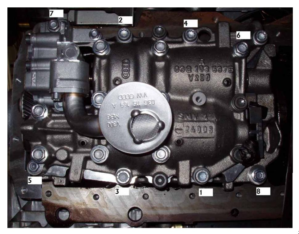
Install all the bolts lightly finger tight. Refer to the picture for bolt sequence numbers.
