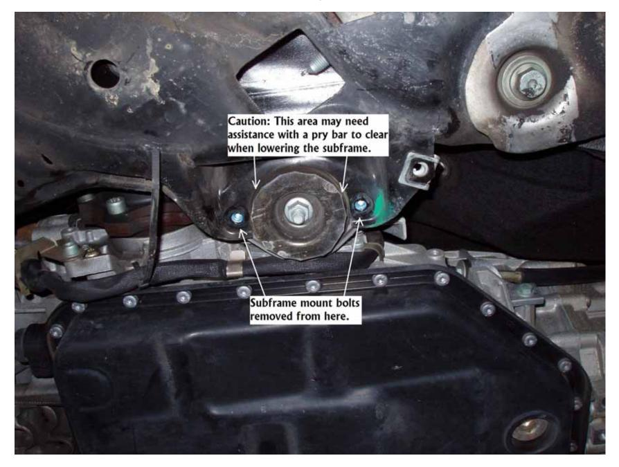
Loosen but do not remove the rear subframe mount bolt. Loosen only enough to allow subframe to hang from the front as necessary when the support is removed.
