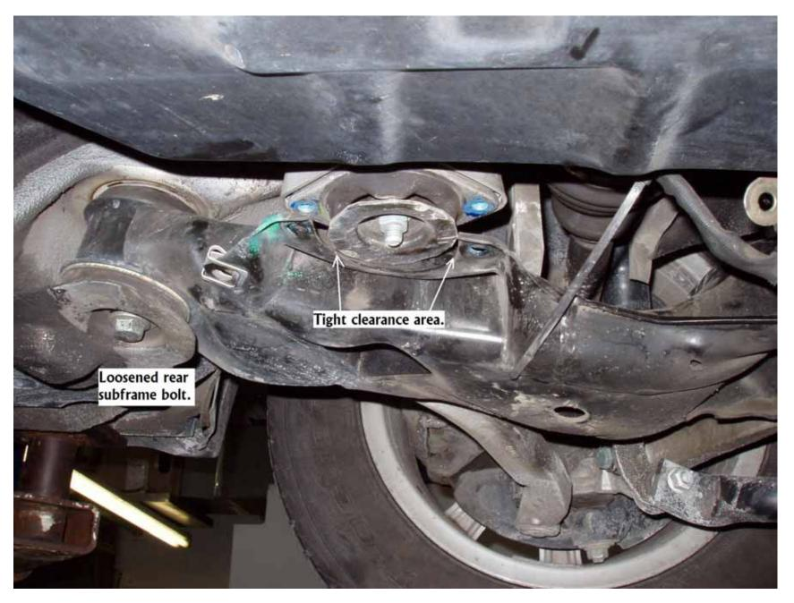
Lower the subframe support slowly and make sure the subframe clears the transmission mounts. The subframe should drop enough so that SST OHTOOL-BJ0002 can be inserted as shown between the subframe and the body.
