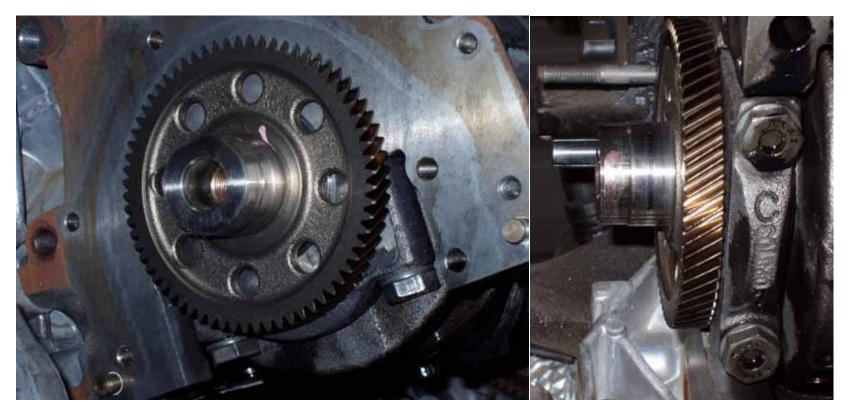
Install the front seal flange without sealant using a couple of bolts.
