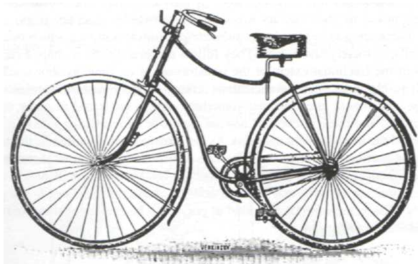
Figure 4.9 The Rover safety bicycle by J K Starley of England, 1885 (McMahon & Graham 1992: 7)
