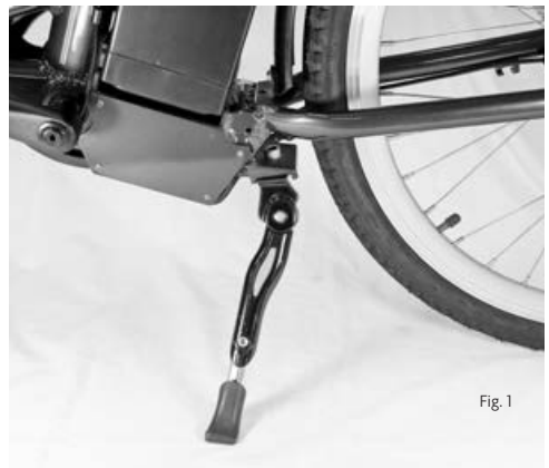
To ride your bike again, push the kickstand anti-clockwise and upward into its retracted position.
