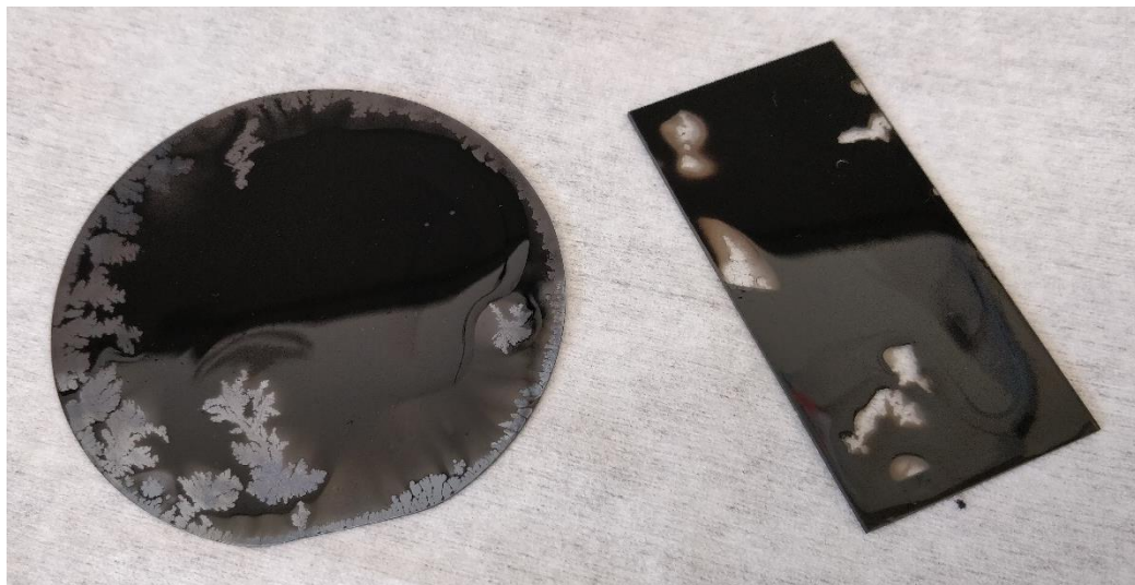
Figure 2.20 Cured samples created by dipping method; silicon wafer (left) and glass slide, G1 (right)
