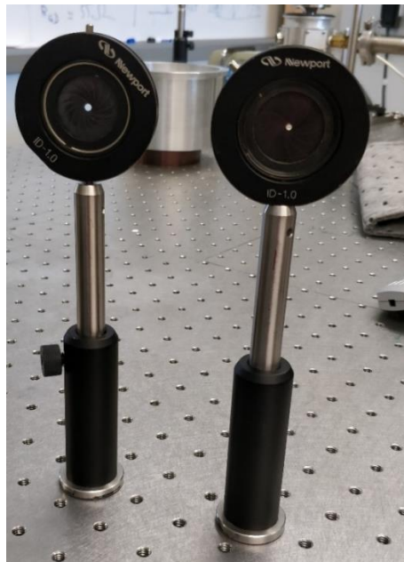
Figure 3.12 Newport ID-1.0 model iris diaphragms used in the measurements for aligning laser beams.
