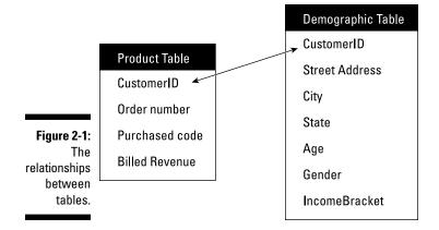
Another aspect of the relational model using SQL is that tables can be queried using a common key (that is, the relationship). In Figure 2-1, the common key in the tables is CustomerID.
