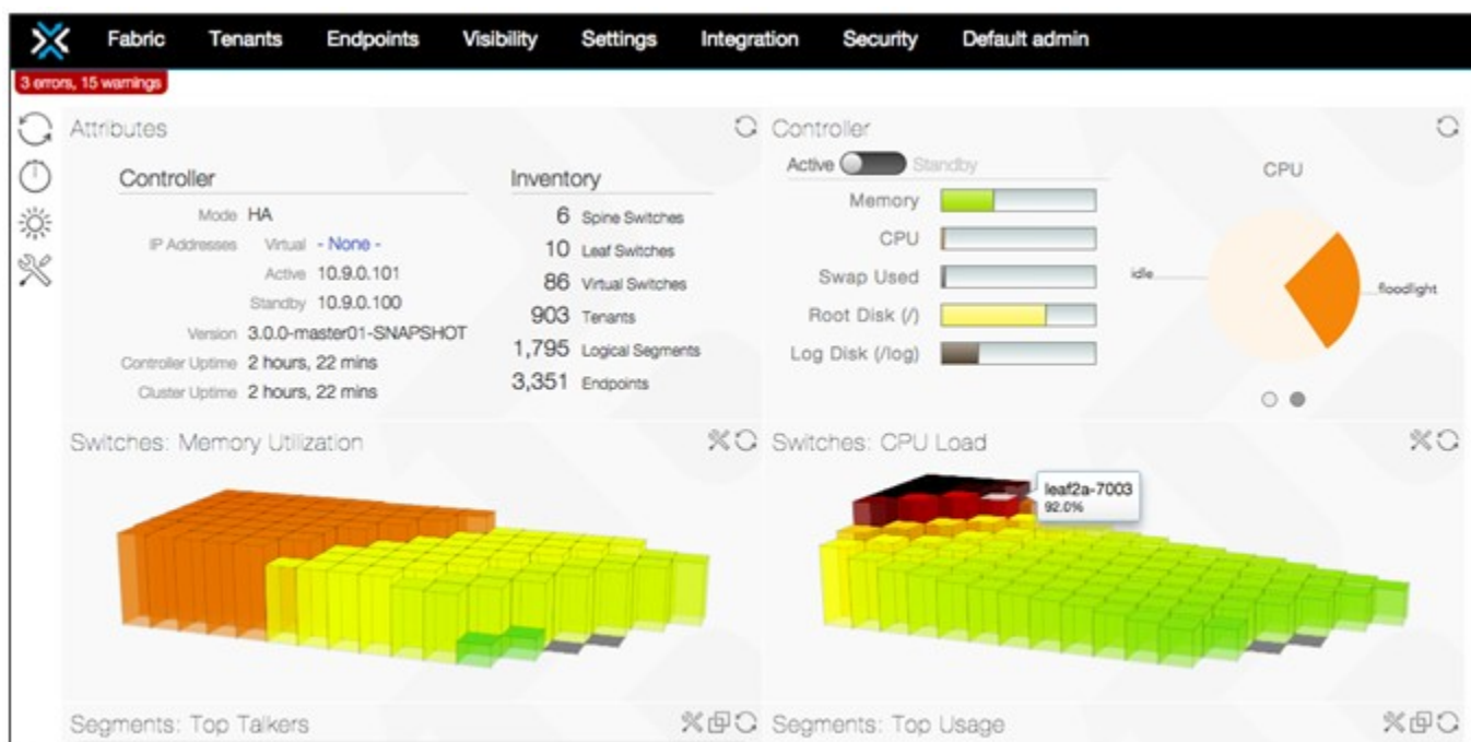
Figure 3. BCF Controller GUI—Current Fabric Status
