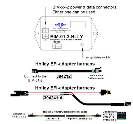
This Bus Interface Module is designed to read engine information from specific Holley EFI kits. The Holley Terminator, HP, Sniper, Dominator and Terminator X and X Max. The module is connected to the Holley EFI through the CAN-bus plug on the EFI harness. Depending on your EFI module you may have a 2-pin or 4-pin CAN connector. We supply EFI adapter harnesses that will allow you to connect with your particular kit.
