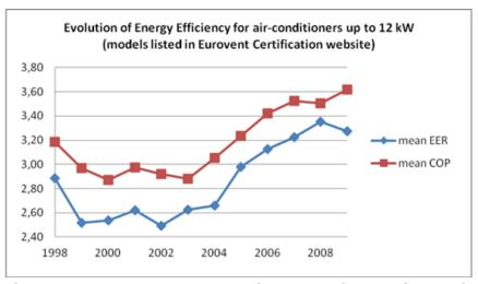
Figure 5. Diagram presents an average performance of AC equipment less than 12 KW in cooling (blue line) and in heating (red line) before and after the new performance labeling regulation 2002. (Eurovent-certified, 20+ manufacturers, more than 1500 product references)
