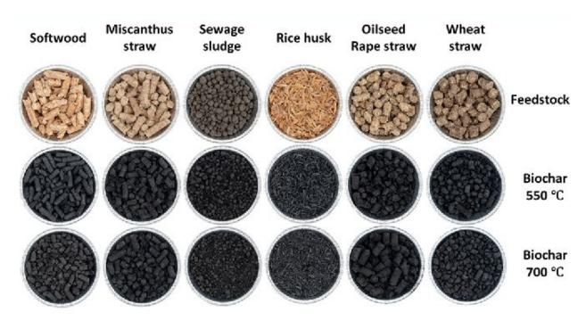
Figure 1. Biochars from different sources, and by pyrolyzation at different temperatures (Mašek, Buss, & Sohi, 2018).
