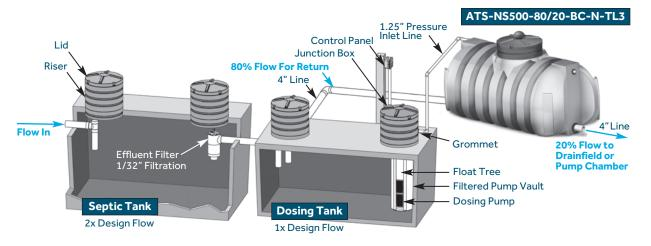
Figure 2 System with Gravity Recirculation Device
