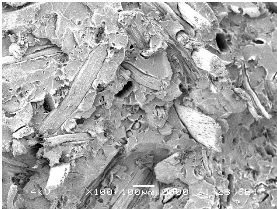
Figure 8 Scanning electron micrograph of PLA-10KF biocomposite at 100x magnification.
