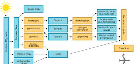
Figure 2: A simplified schematic diagram of different technology pathways to bio-jet fuel
