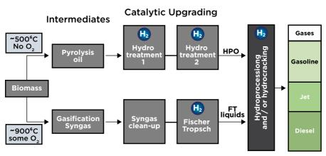
Figure 4: Schematic of thermochemical conversion routes
