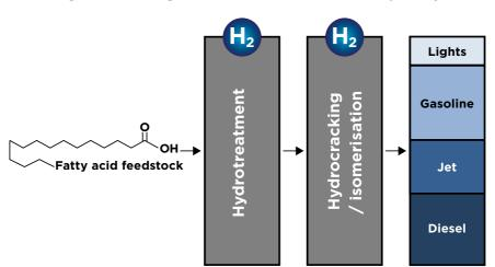
Figure 3: Basic diagram of the oleochemical conversion pathway
