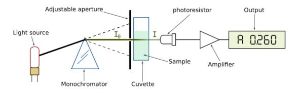
**Figure:** Simple diagram of a spectrophotometer. Image credit: https://commons.wikimedia.org/wiki/File:Spetrophotometer-en.svg
