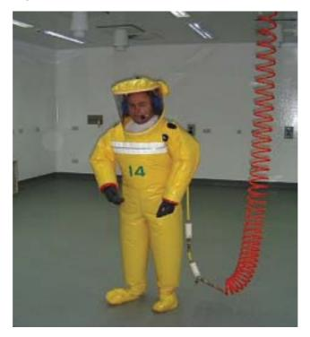
Figure 5: An example of a positive-pressure air-fed suit
