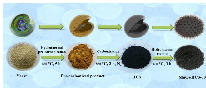
Fig. 1. Schematic illustration of the overall synthesis process for \text{MnO}_2 /HCS-30.
