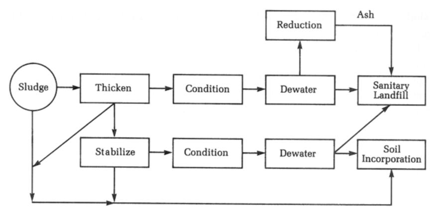
FIGURE 5-31 Basic sludge handling alternatives.
