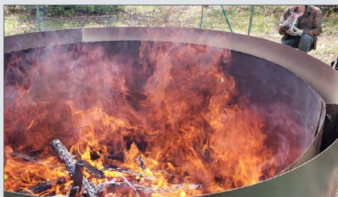
Figure ES-8. The Ring of Fire kiln is portable and used for place-based biochar production (Photo by Kelpie Wilson)
