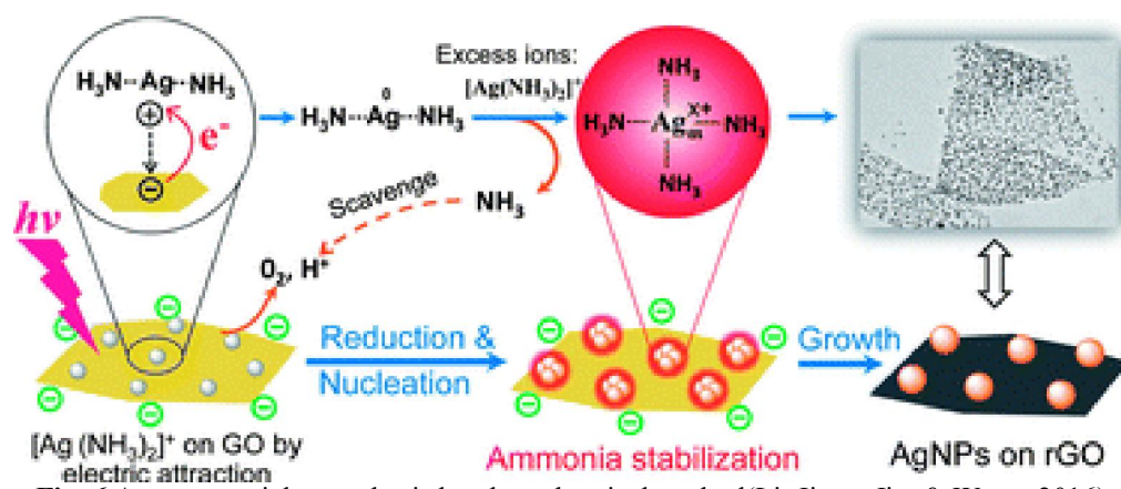
Fig. 6 Ag nanoparticles synthesis by photochemical method(Li, Jiang, Jia, & Wang, 2016).
