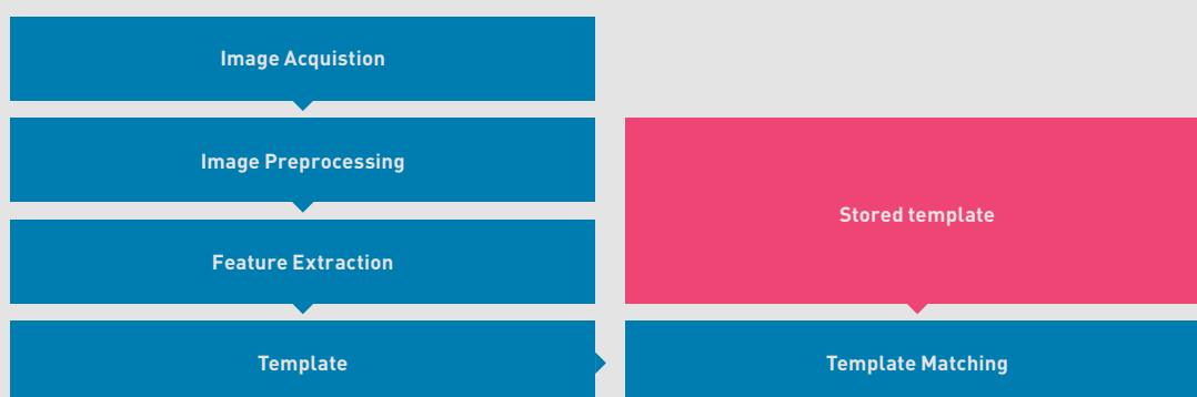
Figure 27. Algorithms for fingerprint recognition
