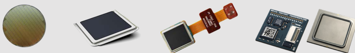
Figure 22. Wafer, LGA, module and stand-alone embedded system.
