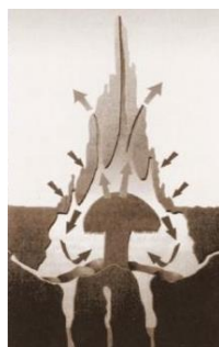
Figure (22): The internal structure of a termite mound with arrows depicting the air flow as an inspiration to self-cooling buildings [6]
