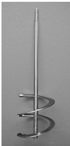
Figure 2.3. The helical ribbon impeller (diameter = 3.30 cm).
