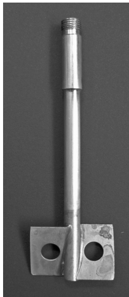
Figure 2.5 The Haake pitched (at an angle of 15 degrees) paddle impeller (diameter = 4.41 cm).
