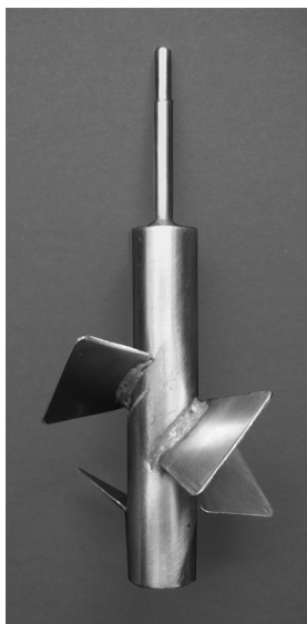
Figure 2.4. The interrupted helical screw impeller (diameter = 5.30 cm).
