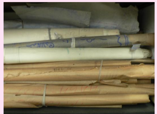
The old patterns were drawn on brown waxed paper by hand and then perforated to allow the ink to pass through onto the fabric.
