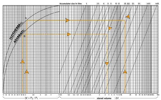
Basic sizing chart for acccumulator used in energy storage.
