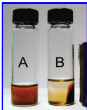
Figure 6. Photographs of (A) \gamma - \text{Fe}_2\text{O}_3 nanoparticles stabilized by 1:1 block copolymer NC1-B2 in cyclohexanone and (B) the same ferrofluid under the influence of external magnetic field.
