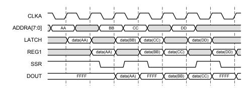
Figure 20: Flow Control Using SSR
