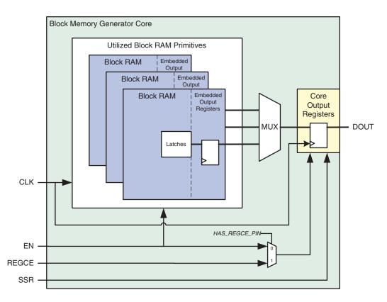
Figure 19: Virtex-4 Block Memory Generated With Both Embedded and Core Output Registers Enabled
