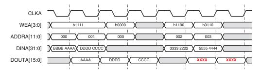
Figure 16: Virtex-4 Write-first Mode Example 3
