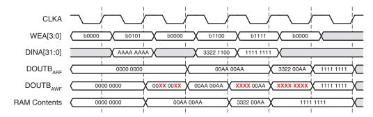
Figure 18: Write-read Collision Example
