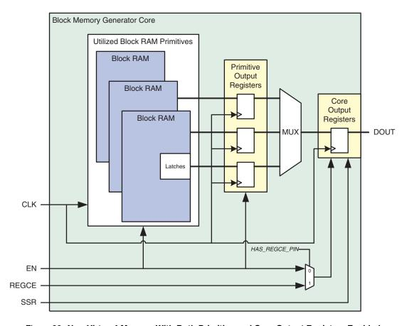
Figure 32: Non-Virtex-4 Memory With Both Primitive and Core Output Registers Enabled
