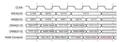
Figure 17: Write-Write Collision Example
