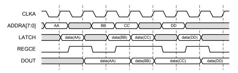
Figure 21: Flow Control Using REGCE
