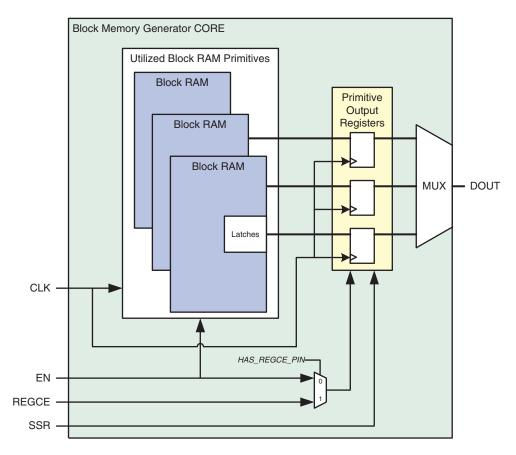
Figure 33: Non-Virtex-4 Block Memory Generated With Primitive Registers
