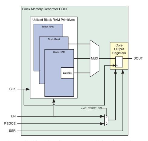
Figure 34: Non-Virtex-4 Block Memory Generated With Core Output Registers
