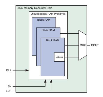
Figure 35: Non-Virtex-4 Block Memory Generated With No Optional Registers
