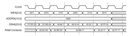
Figure 13: Byte-write Example
