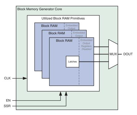
Figure 31: Virtex-4 Block Memory Generated With No Optional Registers
