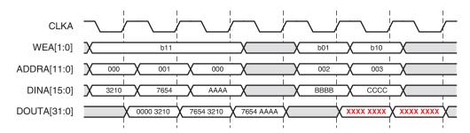
Figure 14: Virtex-4 Write-First Mode Example 1
