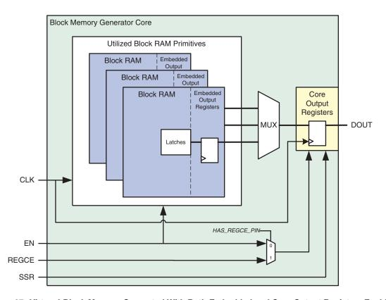
Figure 27: Virtex-4 Block Memory Generated With Both Embedded and Core Output Registers Enabled
