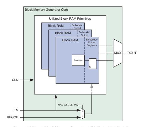
Figure 28: Virtex-4 Block Memory Generated With Embedded Registers
