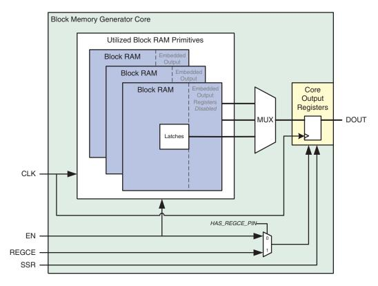
Figure 30: Virtex-4 Block Memory Generated With Core Output Registers
