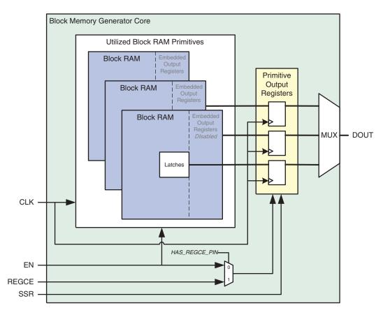
Figure 29: Virtex-4 Block Memory Generated With Embedded Registers and SSR
