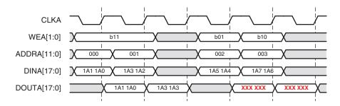
Figure 15: Virtex-4 Write-first Mode Example 2
