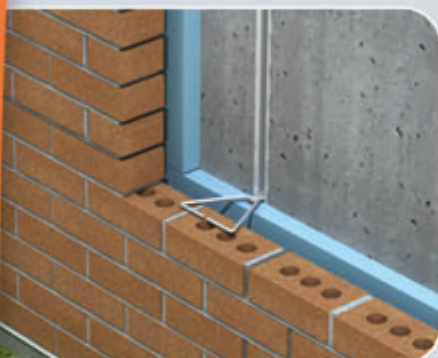
BLT-8 with Dovetail Anchor Slot
