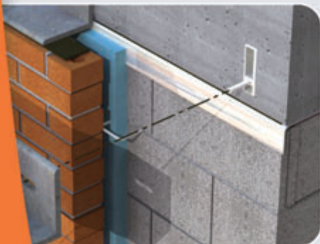
Brick relief angle at concrete beam.
