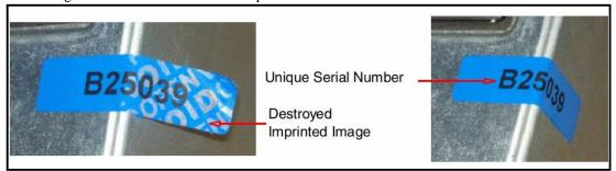
Figure 14 Label Showing Tamper Evidence
