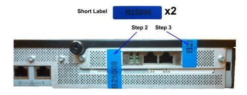
Figure 15 Tamper Evident Label Placement for the NIC Interface Cutout
