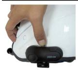
Remove the BlueAnt InterPhone by pushing down the lock as shown and then take out the InterPhone Module in an upward motion.
