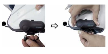
Secure the cord of the Headset Plug(9) inside the helmet. Tuck any extra wire into the helmet. Ensure that only few centimeters of the cord comes out.
