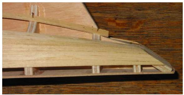
Photo 3: Placing the second planking batten
