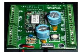
Using the keyboard matrix, I added wires and buttons to allow me to type in numbers. The bluetooth module does an excellent job of button debounce, and basically handles everything for you.
