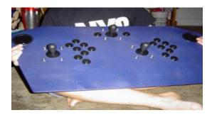
The original control panel had leaf-style switch contacts, meaning that two flexible pieces of metal would be pressed together when a button was pushed or joystick moved. This was sloppy and starting to wear out, so we designed a new control panel that would use microswitch buttons and joysticks. The new control panel worked like a charm, and gave us many hours of Tetris, Zelda, and Super Mario Brothers.
