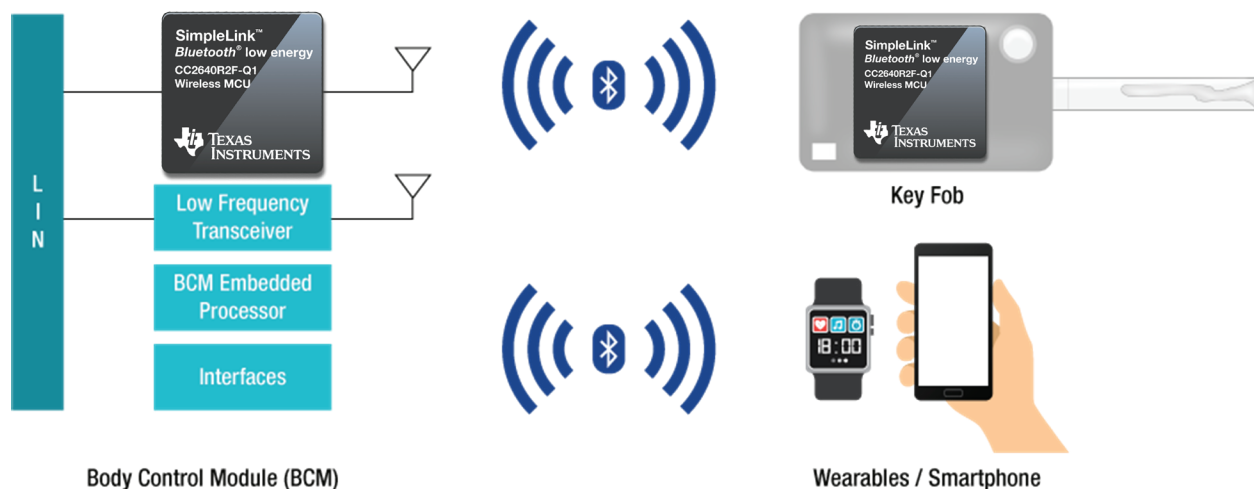
Figure 2. Bluetooth low energy-enabled car access block diagram.
