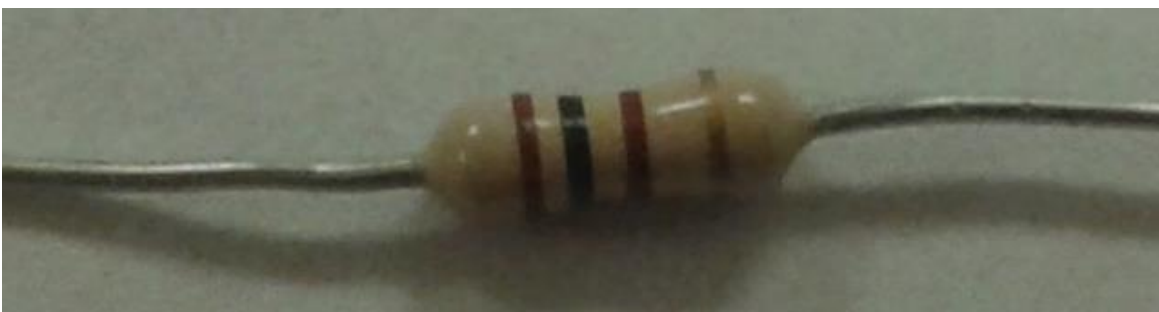
Figure 2: A resistor with the gold band (tolerance band) situated at the right.
