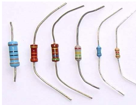
Figure 1: Shows a variety of resistors with different resistive values.
