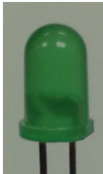
Figure 3: This diagram shows a picture of an LED. Notice the flat edge on the right side, indicating that this is the negative terminal and the left side is the positive terminal.
