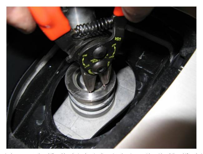
Shifter is then connected to shift rod by placing bearing liners into bearing on either side, sliding shift rod pin through bearing, installing yellow plastic washer, and finally installing the C-Clip:
