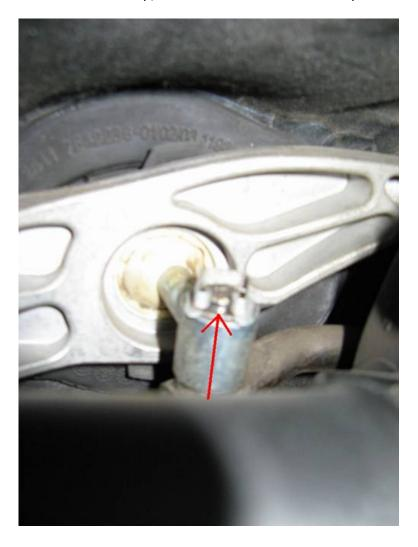
The shifter is also held to the carrier with a plastic collar, it needs to be rotated clockwise to release from the carrier slots it locks into. This plastic collar can be turned by inserting needle nose pliers or a small standard screwdriver into the slots located around the perimeter of the collar. I was able to get the collar turned easily
