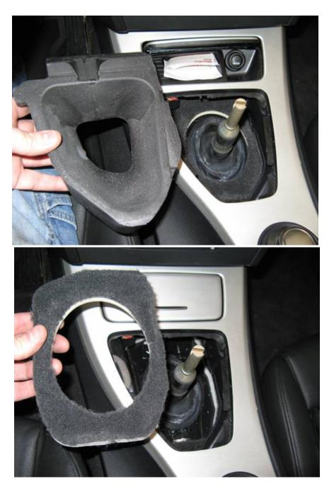
The rubber boot can be carefully removed as well:
