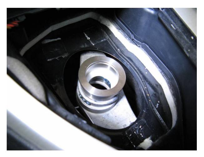
Supplied grease is then applied to shift ball, order of components for installation into carrier from shiftball up should be nylon cup, spring, spring retainer, and snap ring. Also note the slight bend above the pivot ball to the left, the shifter should be installed with this bend towards the driver:
