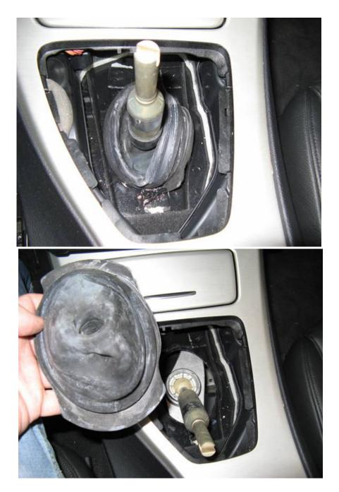
Note in this picture of the bottom of the boot the area that goes around the shifter carrier opening, this can be felt/positioned through the top part of the boot during reinstallation:
