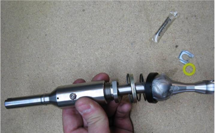
To install shifter in carrier, snap ring pliers are used to insert snap ring into adapter after shifter is placed in carrier:
