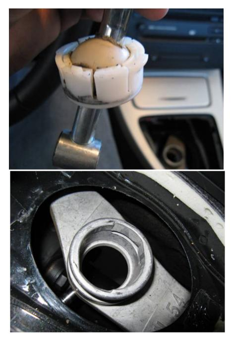
To install the UUC carrier pivot height adapter, the white ring bushing is placed in the adapter with the cup towards the top and Loctite is applied to screw holes on either side:
