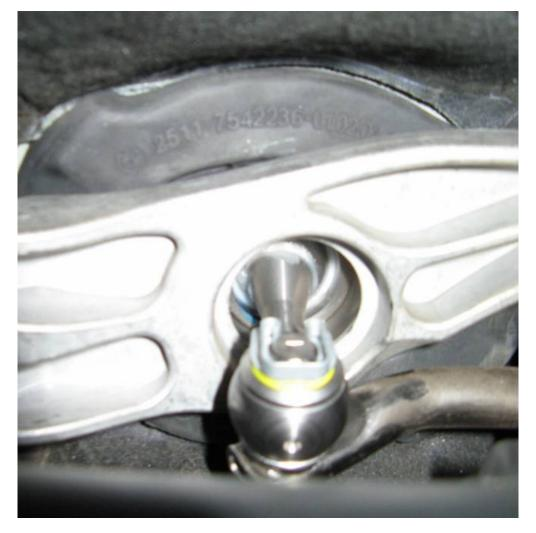
Heat shield is bent back to normal and bolted back up, plastic panel is reinstalled, shifter rubber boot (arrow on boot towards front of car), carpet, foam, shifter leather boot, and knob are reinstalled. When reinstalling the rubber boot, the lower seal for the smaller ring on the carrier around the shifter can be pressed on/around the carrier opening by feel through the rubber boot as the larger lip is press fit into the console body hole.
