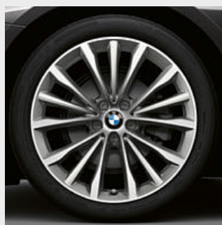
□ 19" light alloy wheels W-spoke style 663 Ferric Grey with mixed tyres and run-flat tyres, gloss-lathed, wheel size front 8J x 19 with 245/40 R19 tyres, wheel size rear 9J x 19 with 275/35 R19 tyres.
