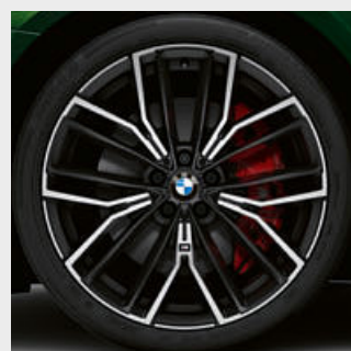
□ 20" M light alloy wheels Y-spoke style 846 M Bicolour Jet Black with mixed tyres and run-flat tyres, gloss-lathed, wheel size front 8J x 20 with 245/35 R20 tyres, wheel size rear 9J x 20 with 275/30 R20 tyres. 2
