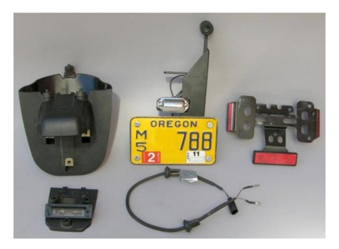
We provide a new license plate bracket that sockets onto the 2nd dowel under the tail section. The flat tab of the license plate bracket bolts on top of the mating flat plate on the exhaust cannister. A  $5/16 \times 18 \times 1$  bolt holds the two together.
