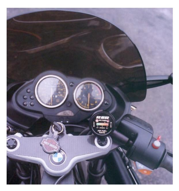
When you get around to Installing the RSR Air Fuel Ratio Gauge, cut the O2 wiring sheath back and either use Scotch Lock the Green Wire from RSR meter to the black signal wire. Installation instructions for the RSR Air Fuel Ratio Gauge are downloadable from RB Racing's website rbracing-rsr.com:
