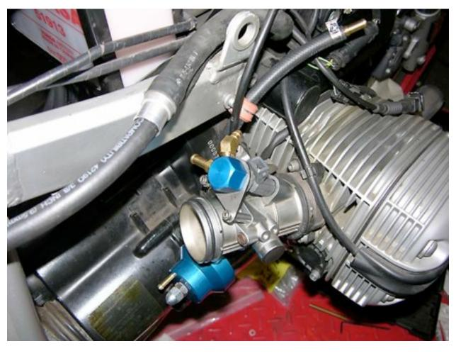
Fuel System...Right Throttle Body Fuel Rail
