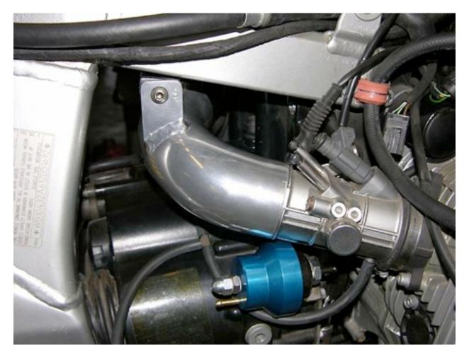
Right Zero Restriction tube is the shorter of the two. Powder coated brackets provided bolt to the inside of the frame rail on the oem 8mm studs. The tubes bolt to the outside of these black brackets with the stainless steel button head screws provided.
