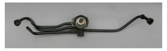
The fuel lines and injectors can be removed along with the oem regulator assembly. Leave the lines attached to the injector feed caps as we are going to replace all these lines.
