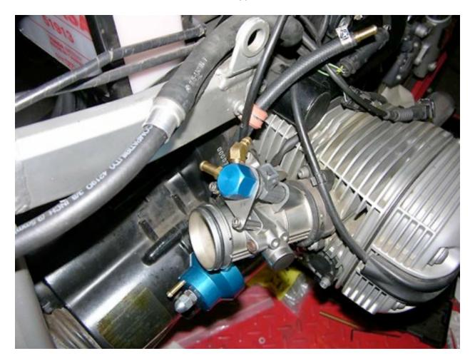
The 1/4 return line goes from base of regulator (12mm nut end) to tank return line. Use  $1/4 \times 5/16$  machined reducer/coupler. Note the clamps are two sizes, one for 1/4 and one for 5/16.
