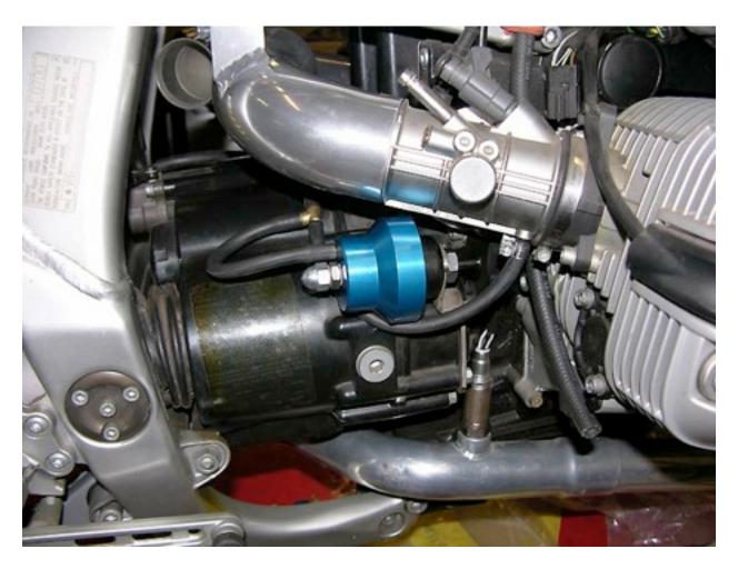
A vacuum line connects the two throttle bodies to the top of the Bosch Billet Fuel Regulator. Two clamps are provided for the hose to throttle body connections. No clamps are needed on the tee. Manifold pressure will track fuel pressure 1:1 unlike the oem system which will slightly lower fuel under vacuum and raise fuel delivery under low vacuum (full throttle) compared to the non-referenced oem regulator.
