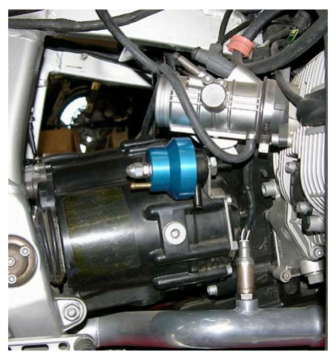
Regulator mounts on right side of transmission just above the new O2 sensor location. The return port next to the 12mm mounting nut faces forward. It must be set to 46.5 psi (3.2 Bar). Oem Pressure is 43.5. To adjust pressure remove acorn nut, loosen lock nut and use screwdriver. CCW to lessen. CW to increase. Fiber seal washers under both jam and acorn nut.
