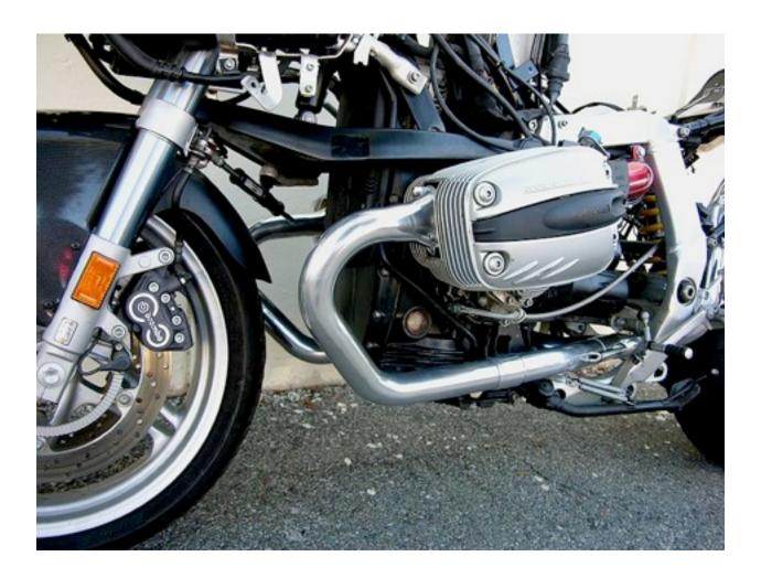
The RB Racing LSR 2-1 Black Hole exhaust simply sockets into the front ports (reuse the oem gasket)....and it sockets or slides onto the dowels under the tail section. Springs are provided for the left side slip and for the muffler.
