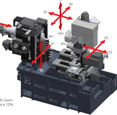
Superimposition control allows simultaneous cutting with two tools at the main spindle (SP1), or with three tools when the sub spindle (SP2) is included, shortening cycle times.
