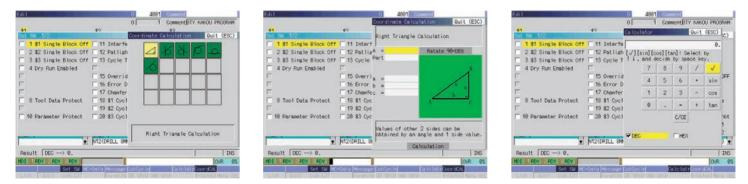
The coordinate calculation function and calculator function incorporated in the NC unit can be used for complex intersection point calculations.
