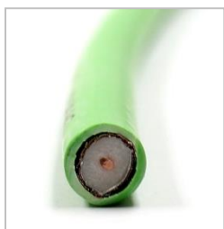
cut with cable shear
