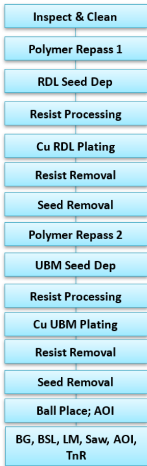
Figure 3. WLCSP manufacturing process flow.
