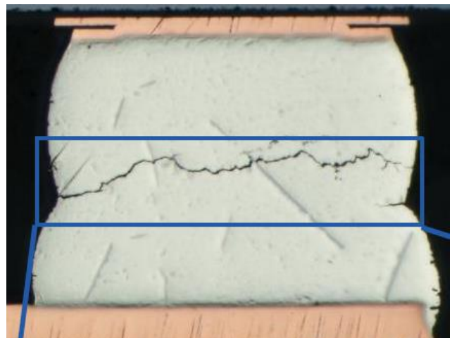
Figure 18. Leg 5 (5S mold + SACQ ball) solder crack.
