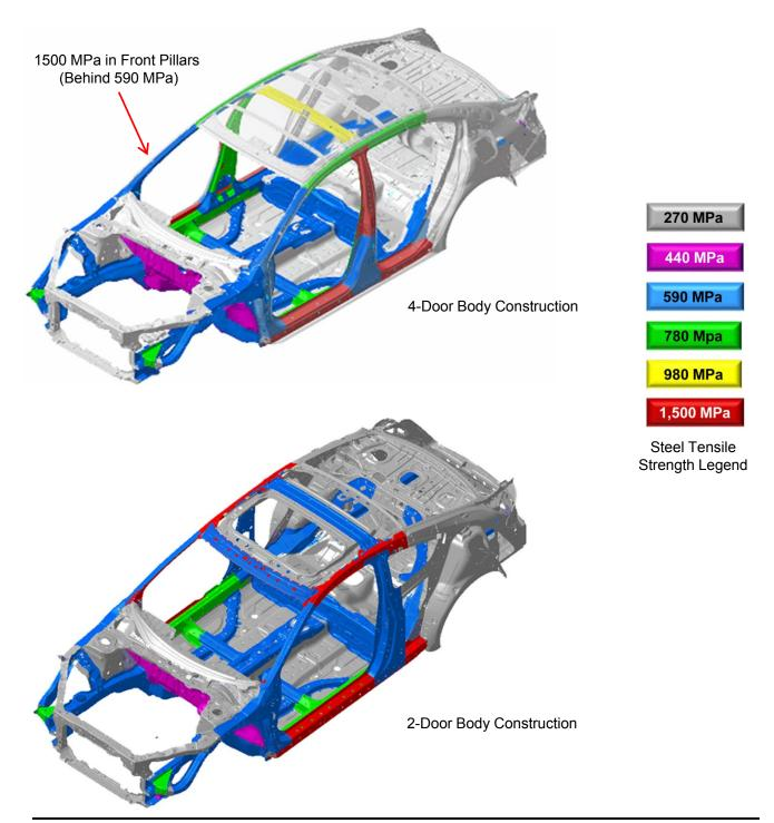
**1,500 MPa (HOT STAMP) STEEL LOCATIONS**1,500 MPa steel is stronger than ordinary steel, so it can help protect vehicle occupants while reducing overall vehicle weight to improve fuel efficiency.
