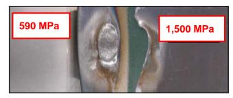
Tensile Test Results of MAG-Welded 1,500 MPa Steel
