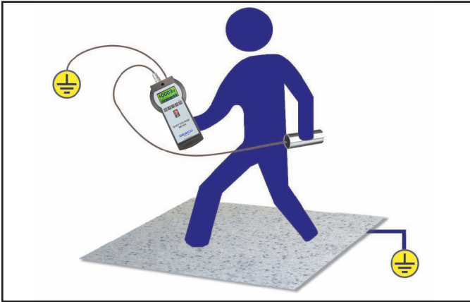
Figure 3. Setup of the Body Voltage Meter
