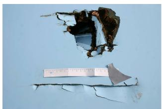
Figure 2. Damage to left engine cowling (close-up view)
