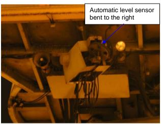
Figure 3. Damage to aerobridge automatic level sensor
