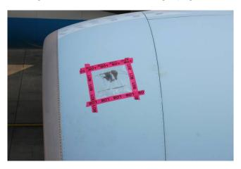
Figure 1. Left engine cowling damage location at 1 o'clock position
