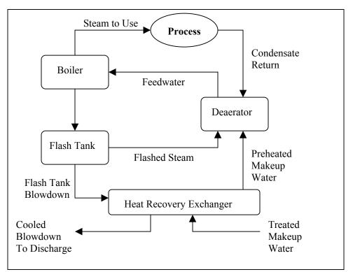
Schematics of a Flash Tank - Heat Exchanger System
