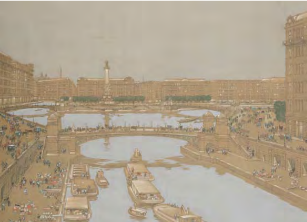
Plan of Chicago plate 107, 1909. “View looking north on the south branch of the Chicago River. Showing the suggested arrangement of streets and ways for teaming and reception of freight by boat, at different levels.”
