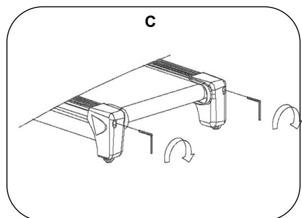
**NOTE:** When properly tightened, you should be able to peel the very edge of the side of the belt up approximately 2 inches. However, this is a rough reference and not all treadmills are the same. Some treadmills that have longer belts may give different measurements for correct belt tightness. Simply, if the belt begins to slip during use, this is an indication that the belt still needs tightening.
