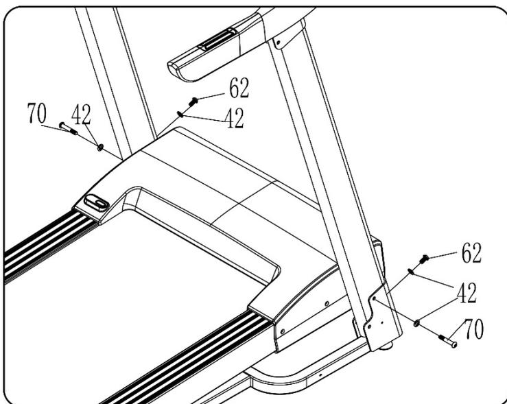
1. Use 5# Allen wrench (10) to secure right upright onto base frame with bolt (70), bolt (62) and 2x lock washer (42).
