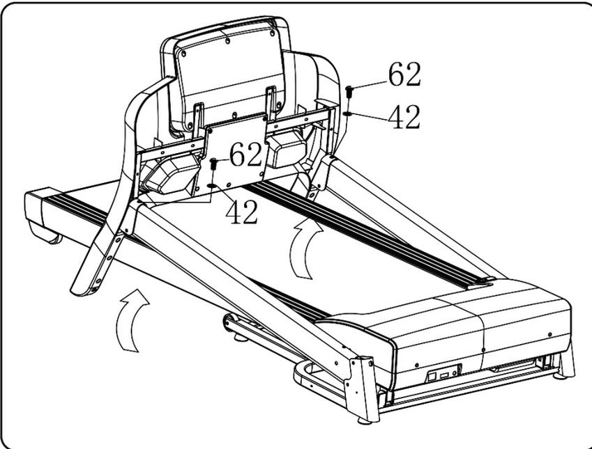
1. Hold the computer frame and use the 5# Allen key (10), bolt (62) and lock washer (42) to secure the computer frame onto the right and left upright. Refer to image.
