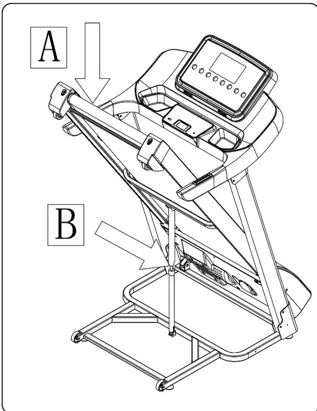
Whilst supporting position (A) with our hand, gently push position (B), the marked area on the air pressure bar, with your foot. The base frame will descend automatically. (Please keep people and any pets away the machine during descent)
