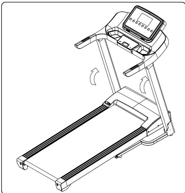
1. Position the display according to the illustration.
