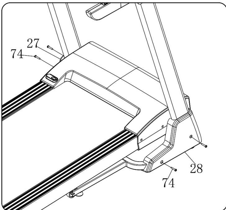
1. Use wrench w/screwdriver (12) and secure the right base cover (28) to the right upright and base frame, using bolt ST4.2\*19 (74).
