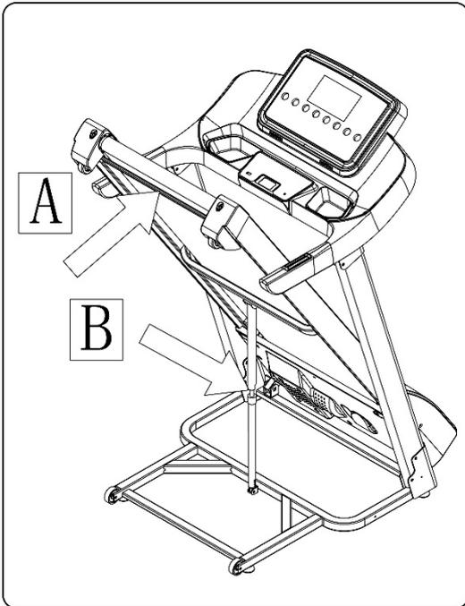
Place your hand on position (A), then pull up the base frame until you hear the click sound emitted when the air pressure bar (B) is locked into the round tube.
