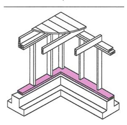
This illustration shows earthquake forces pushing on the mudsill and the placement of bolts that prevent movement.
