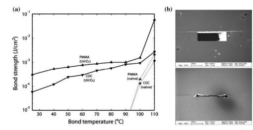
Fig. 9 a Bond strength of PMMA and COC substrates following 24 min UV treatment, compared with native polymer surfaces, and b SEM images of 500  $\mu$ m wide, 180  $\mu$ m deep PMMA microchannels bonded at 60°C following UV/ozone treatment (*top*), or at 100°C with no treatment (*bottom*). While substantial collapse of the channel is
