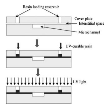
**Fig. 3** UV-curable adhesive application using capillarity-mediated resin introduction (Lu et al. 2008). Copyright Wiley-VCH Verlag GmbH & Co. KGaA, reproduced with permission
