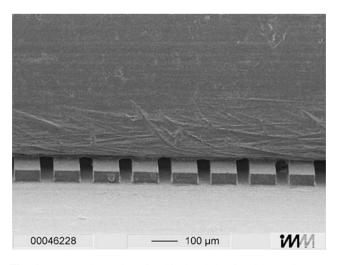
**Fig. 6** PMMA electrophoresis chip bonded using isopentylacetate deposited by solvent stamping (Griebel et al. 2004). Reproduced by permission of The Royal Society of Chemistry
