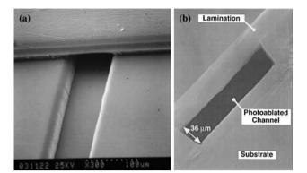
Fig. 4 Laminate film sealing based on **a** pressure sensitive film (Huang et al. 2007), and **b** thermal lamination film (Roberts et al. 1997) (copyright Wiley-VCH Verlag GmbH & Co. KGaA, reproduced with permission)
