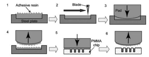
**Fig. 2** Adhesive application using a contact printing process. Adhesive was poured on steel plate with a hollow and spread over the plate using a blade (step 1, 2). Adhesive was applied on the silicon rubber pad (step 3, 4). The adhesive on the silicone pad was deposited on the
