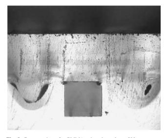
**Fig. 8** Cross-section of a PMMA microchannel ca. 500 µm square sealed by ultrasonic bonding, with deformed energy concentration structures evident on either side of the channel opening (Trucken-muller et al. 2006a). Copyright Elsevier, published with permission
